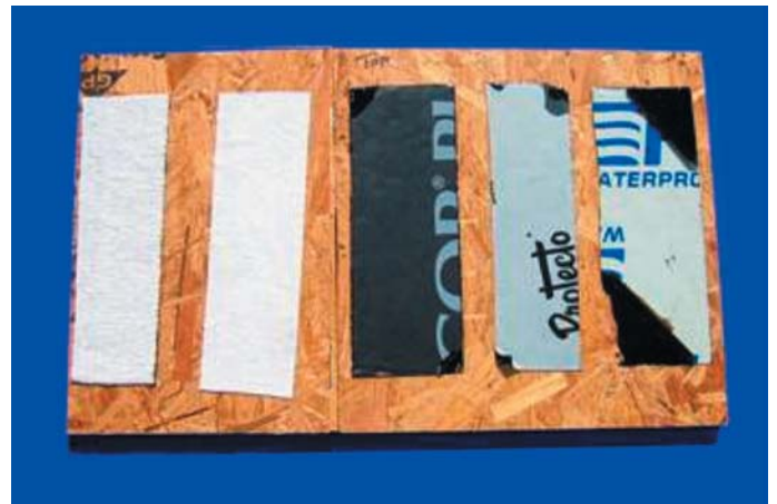
Figure 11: Self-adhered flashing samples after aging 24 hours at 160°F. Note top sheet delamination for asphalt
