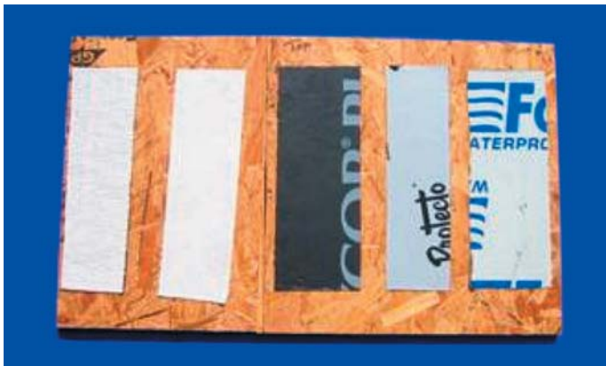
Figure 10: Flashing samples on OSB before aging. Two on left are DuPont butyl based, three on right are asphalt based.
