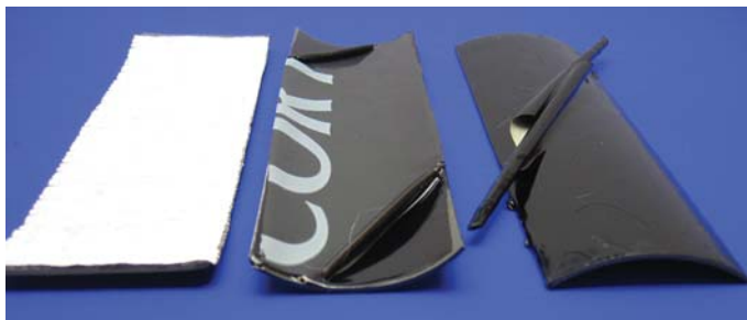
Figure 14: Closeup shot of samples aged 7 days at 160° F on vinyl strips. The sample on the left is DuPont™ FlexWrap™ and the ones on the right are asphalt based.
