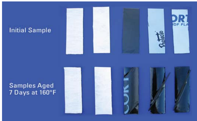
Figure 13: Self-adhered flashing samples on vinyl strips, before and after heat aging 7 days at 160°F
