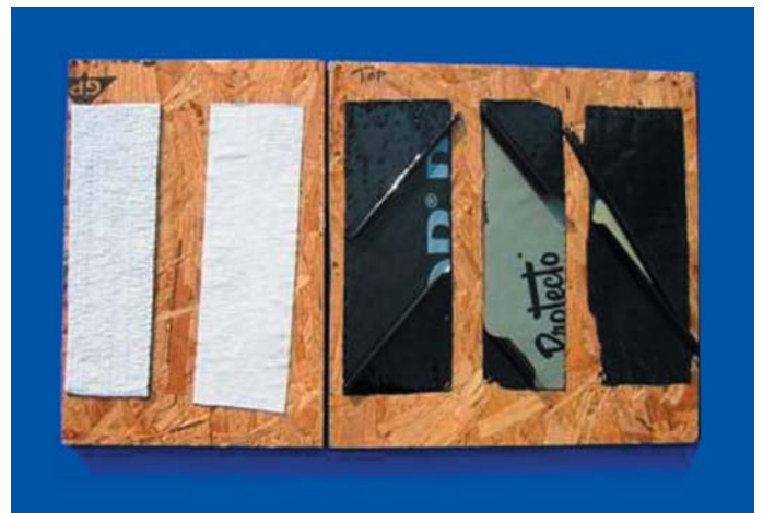
Figure 12: Self-adhered flashing samples after aging 7 days at 160°F.
